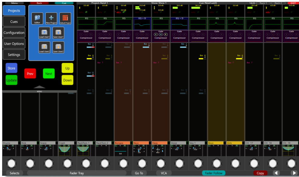
97: CM-Editor: The Control Screen window is accessed by selecting the Menu button at the top left of the displayed. This gives access to the menu structure that is found on the console's 6.5" physical displayed, along with the Back and Cue buttons.
