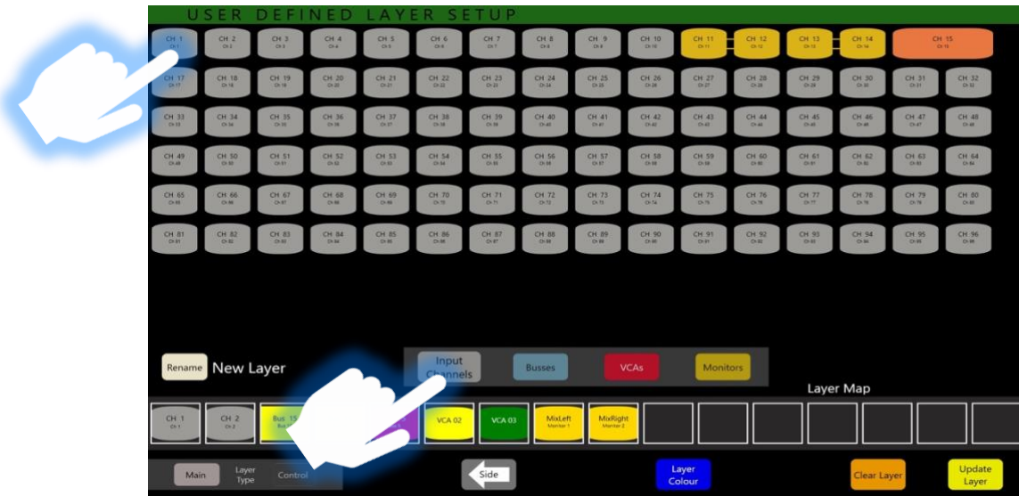
58: User Define Layer Setup: Select Input Channels, then select the input to be added to the customer layer
