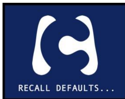
42: Recall defaults – the unit will now continue and reset to factory defaults
